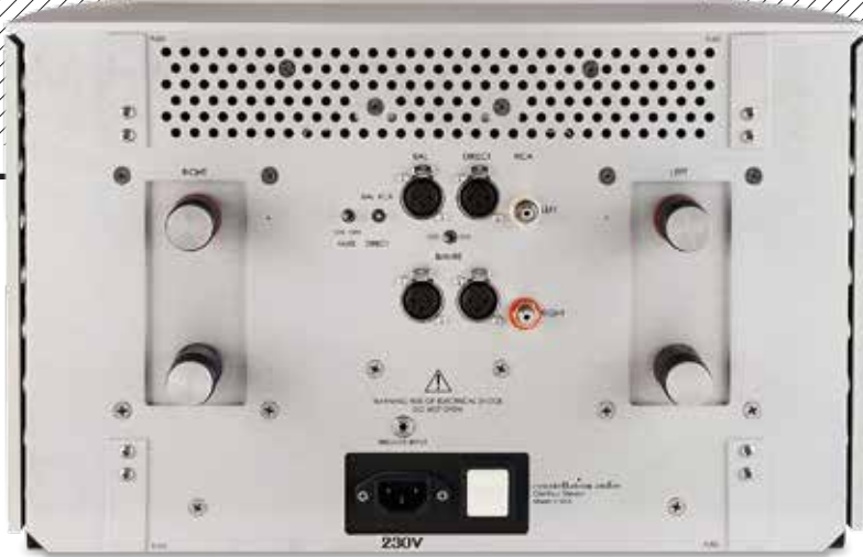
ABOVE: There are two balanced (XLR) inputs per channel – one high gain, the other ‘Direct’ lower gain [see boxout, p67] – and one single-ended (RCA) input, selected by a small toggle switch. The beefy speaker cable terminals are best suited to spades
